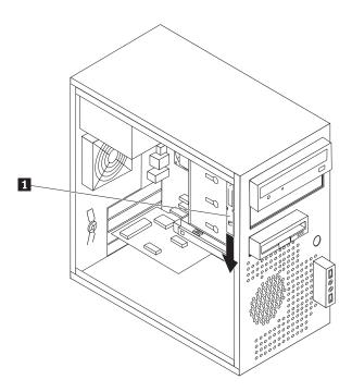
Figure 13. Locating the spare retainer
